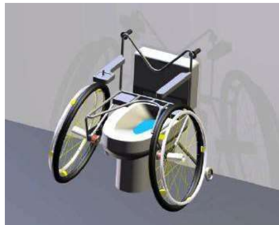
Final simulation of wheelchair coupling with the toilet.
