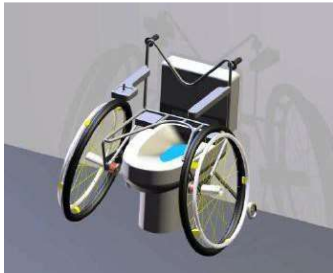
Final CAD Design of wheelchair coupling with the toilet.
